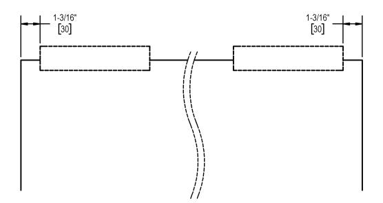
Please note: When end stops are used, the carriages must be indented by at least 1-3/16" [30 mm]. A flush installation of the carriages as per step 5 of the mounting instructions is therefore no longer possible. When end stops are used in combination with a damping mechanism on both sides, the door width increases by 2-3/8" [60 mm] respectively.
